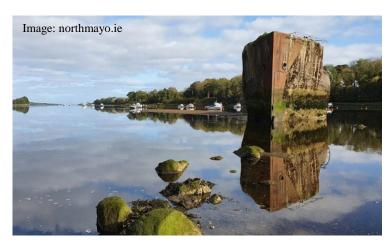
However, by 1924 company had ceased operations and all its vessels were left mothballed on the River Tyne. The SS Crete Boom was laid up on the River Wear for a number of years before being sold for dismantling. It was stripped of its metal parts leaving only the concrete hulk of the boat.
